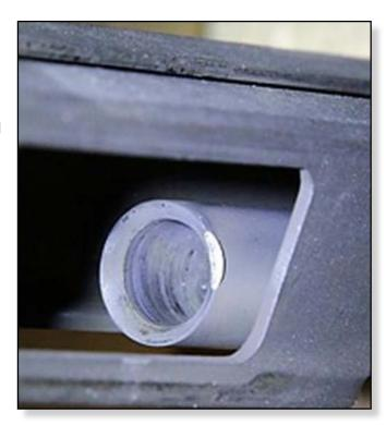
**Is your barrel chamber within spec?** Take the upper receiver off the lower and remove the bolt. Insert an unfired 9MM round upside down into the chamber. It should go in no more than halfway. If it goes in any further, then your barrel chamber is too loose and may cause "short stroking" or failures to eject or strip rounds.
