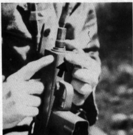
1. Fast, simple disassembly procedure. Depress upper-receiver retaining pin latch.
