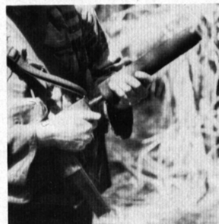
7. Easy attachment/detachment of sound-suppressor (silencer) to M10 allows weapon to fulfill many roles.
